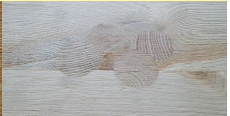
Falling out knots removed, plugs pasted
