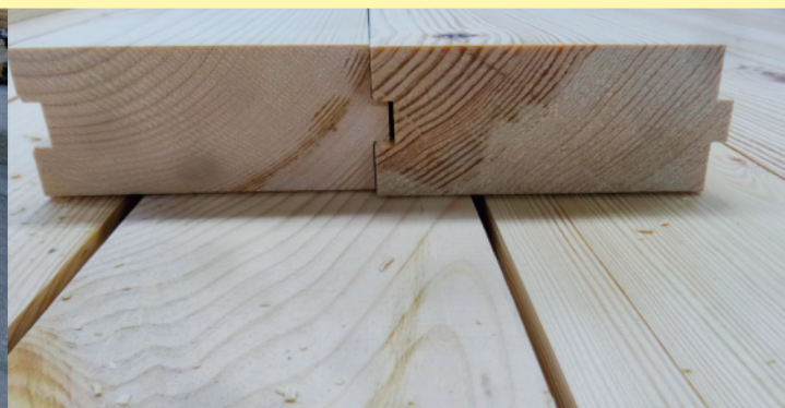
Boards connected by tongue-groove
