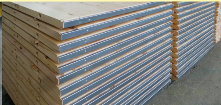
Boards glued and screwed with three screws with springs to compensate
